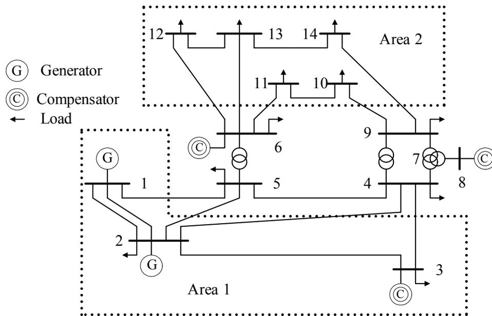
Fig. 3. IEEE 14-node test model
