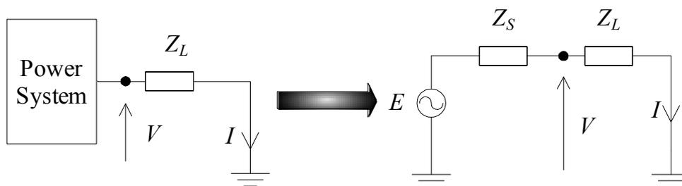
Fig. 1. Power system representation as Thevenin equivalent
